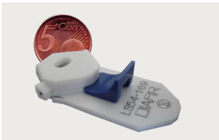
Fig. 5 Single-use mid-infrared medical sensor
